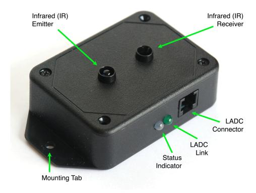
INFRARED EMITTER - Sends out encoded infrared signal that bounces back to the sensor to indicate the presence of a person or an object.
